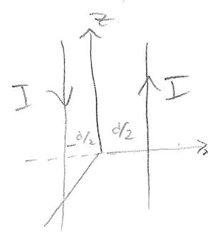
Let's start by thinking of just one current-carrying wire flowing up thru  $x, y = 0$ . Then we'll shift it right to  $x = d/2$ , and add a second wire in at  $x = -d/2$  by superposition.
