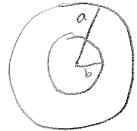
$a-b \ll a$  (Not drawn to scale).The modes are characterized by  $(\nabla_{\perp}^2 + \gamma^2) \Psi(p, \phi) = 0$
